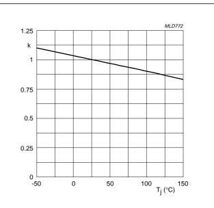
$$k \, = \, \frac{V_{GS(th)} \, \, at \, T_j}{V_{GS(th)} \, \, at \, 25 \, \, ^{\circ}C}. \label{eq:kappa}$$
