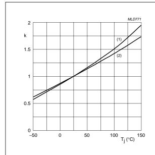
$$k \, = \, \frac{R_{DS(on)} \, \, at \, T_j}{R_{DS(on)} \, \, at \, 25 \, \, ^{\circ}C} \label{eq:k_scale}$$
