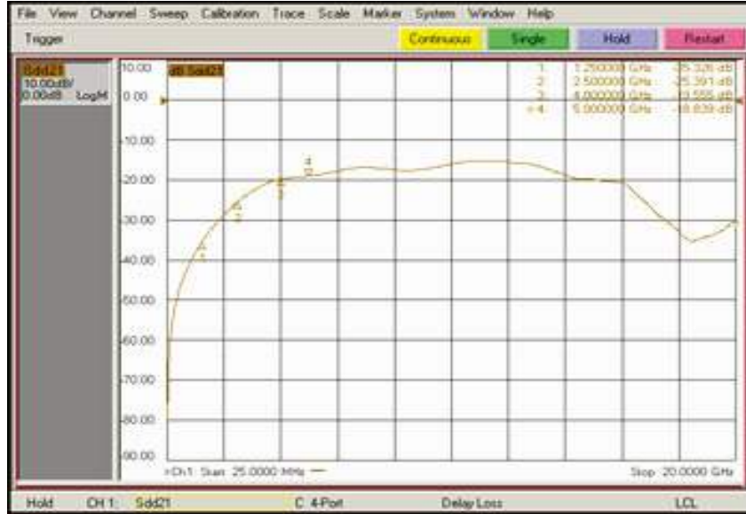
Differential Off Isolation
