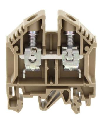
Ex feed-through terminal ATEX-certified, Screw connection, Mounting type:Mounting rail TS 35/7.5 and TS 32, Rated cross-section: 16 mm², Width: 12 mm, Colour: Beige
