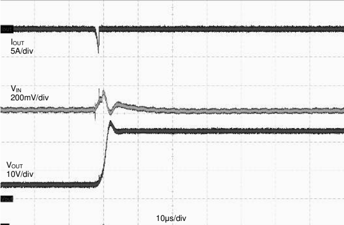
Reverse-Voltage Response V_{IN} = 5\text{V} , Supply 24V to OUT Port
