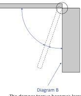
The damper torque becomes larger, preventing the lid from closing completely
