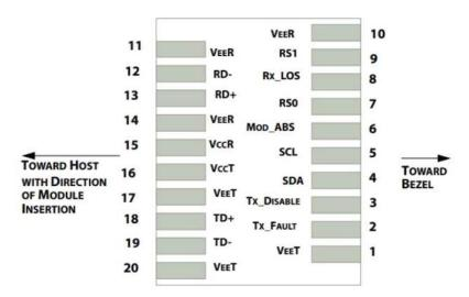
**Electrical Pin-out Details for SFP**
