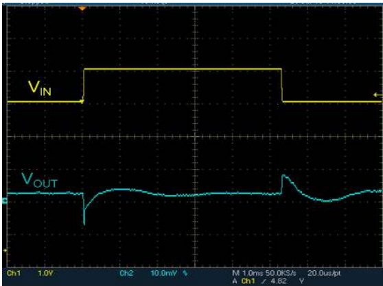
Figure 13. Line transient (no load)
