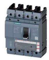
circuit breaker 3VA5 UL frame 250 breaking capacity class M 35kA @ 480 V 4-pole, line protection TM210, FTFM, In=175A overload protection Ir=175A fixed short-circuit protection Ii=10 x In N conductor protection 100% without connection
