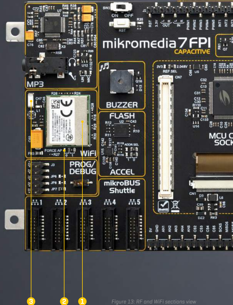
Figure 13: RF and WiFi sections view
