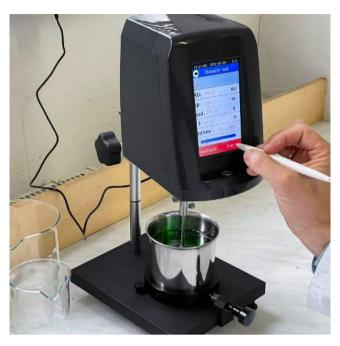
Viscometer / viscosity meter with PC interface / Optional ISO factory certificate / Touchscreen / Measuring units KU, cP, g / Measuring range 40.2 ... 141 KU / Height-adjustable stand mount / For measuring the viscosity of liquids / Overload protection / Optional software
