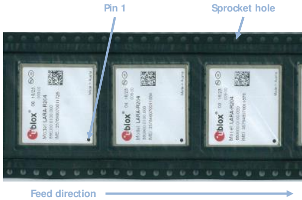
Figure 5: Orientation for LARA-R2 series modules on tape
