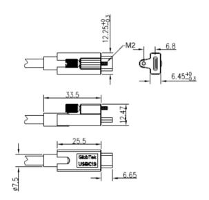
Mates with GlobTek USB Type C cables with 2 screws.
