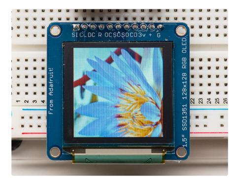
To make new bitmaps, make sure they are less than 128 by 128 pixels and save them in 24-bit BMP format! They must be in 24-bit format, even if they are not 24-bit color
