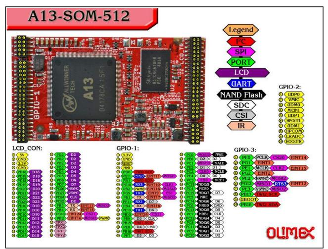
To keep the form factor as small as possible the GPIO connectors have 0.05" step.
