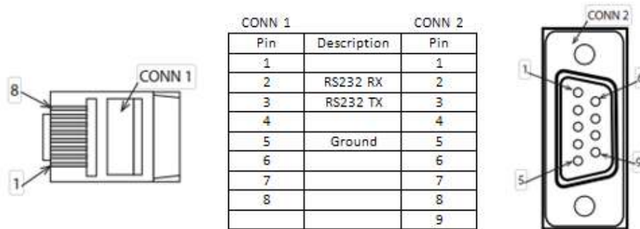
Figure 22: Serial Cable Pinout
