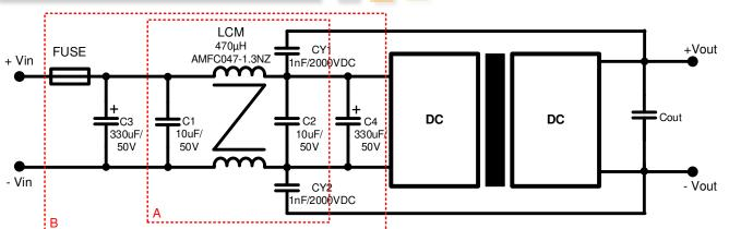
Notes:Part A for EMI filtering and Part B is used for EMS test.
