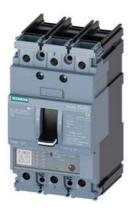
circuit breaker 3VA5 UL frame 125 3-pole, starter protection TM120M, AM, In=110A without overload protection short-circuit protection Ii=5...12 x In cable connection on both sides
