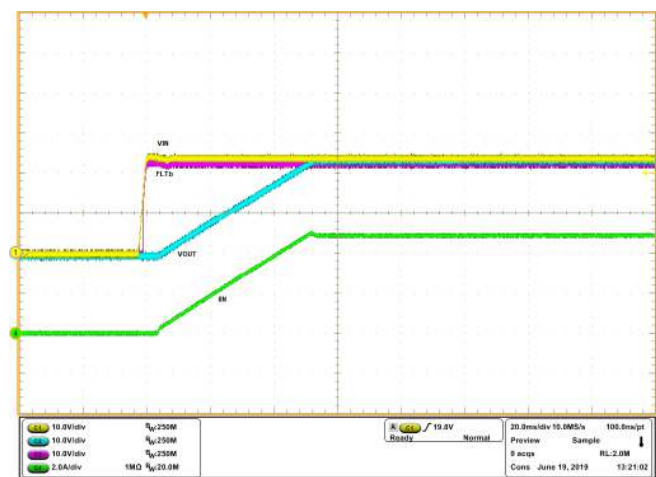
Figure 4. TPS2663-166EVM Startup for CH2 ( V_{IN} = 24\text{ V} , I_{LIM} = 6\text{ A} , R_{OUT} = 4.8\ \Omega , MODE = GND)
