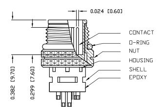
858-012-103RLSY 3 = BRASS/TIN (B/T) SHELL & BRASS/NICKEL NUT -= STAINLESS STEEL (SS) SHELL & NUT T = B/T SHELL / SS NUT= GOLD FLASH -
