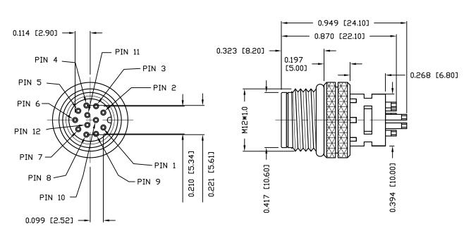
NOTE: MATERIAL HOUSING: PBT UL94V-0, BLACK CONTACT: **BRASS** NUT: **BRASS D-RING**: **EPDM** SHELL: **BRASS FINISH** CONTACT: GOLD PLATED **DVER 50u" NICKEL** NUT: NICKEL PLATED SHELL: BRIGHT TIN PLATED **ELECTRICAL** RATED CURRENT: 1.5A 30V RATED VOLTAGE: INSULATION RESISTANCE: 100 MOhms MIN. CONTACT RESISTANCE: 10 mOhms MAX. WATER PROOF: IP67 **ENVIRONMENT OPERATION TEMPERATURE:** -40°C TD +85°C MAX WIRE AWG: 24
