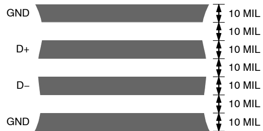
Figure 17. Arrangement of Signal Tracks
