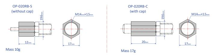
Note: When attaching, make sure that the side without a bearing chamfer is the impact surface.
