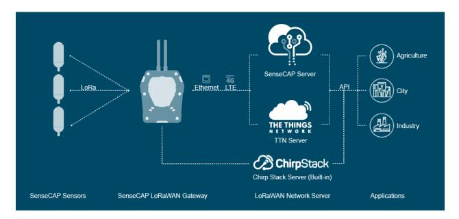
SenseCAP Sensor + Other LoRaWAN Gateway Architecture
