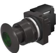
30mm BlackMax, Epoxy Coated Corrosion Resistant Complete Metal Unit Illuminated Push-Pull Operator Full Voltage, 120V AC/DC Incandescent Lamp Mushroom Head Cap Small 1 3/4" (44.5 mm) Metal, Black with Green Lens 3 Position Pull-Momentary/Push-Maintained UL Listed, CSA Certified NEMA 1,3,3R,4,4X,12,13 & Automotive Standards
