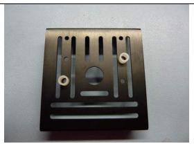
Using a screw, nylon washer, and hex nut; connect the PING))) module to the plate. Do not tighten the screws all the way until you have adjusted the PING))) to make sure it is being installed straight.
