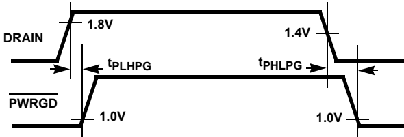
FIGURE 4A. DRAIN TO \overline{\text{PWRGD}} TIMING (ISL6140)
