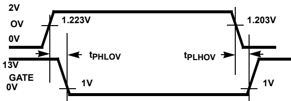
FIGURE 3A. OV TO GATE TIMING
