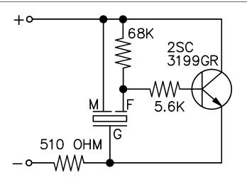
Notes: 1. The current consumption and the sound pressure level are measured by using the recommended driving circuit shown above.
