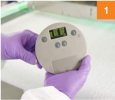
1 Validate UV cure chamber conditions.
