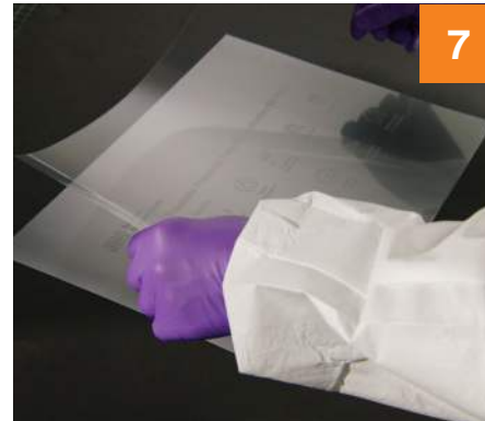
7 Part can be bonded immediately or a release liner can be added.
