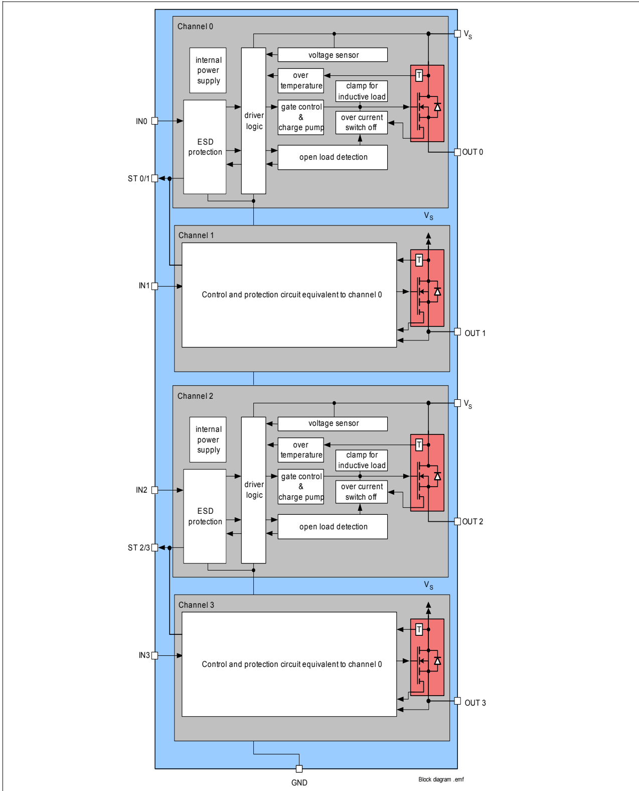
Figure 1 Block diagram for the BTS4130QGA
