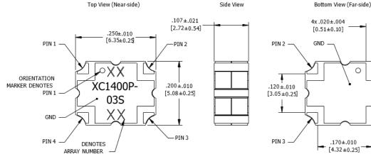
Dimensions are in Inches [Millimeters] XC1400P-03S Mechanical Outline Rev D
