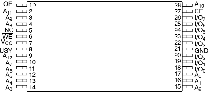
TSOP Package (8 mm x 13.4 mm) (H13)
