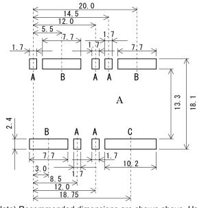
Note) Avoid wiring patterns directly underneath the converter (the first layer). Since this product uses a standard through-hole board, a pinhole on the resist may cause problems.
