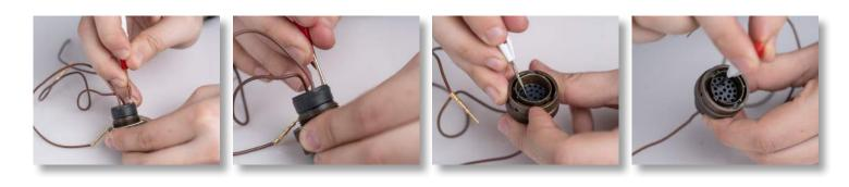
This tool is perfect for inserting and extracting size 20 front release contacts made by most manufacturers. This insertion tool features the following:
