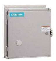
Mechanically held lighting contactor, Contactor amp rating 20Amp 0NC  $\_$  2NO poles, 265-277V 50/60HZ coil, Non-combination type, Encl NEMA type 4X 304 S-steel Water/dust tight noncorrosive
