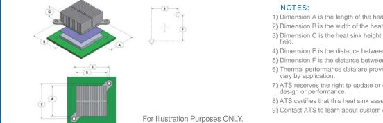
1) Dimension A is the length of the heat sink in the direction of the flow.
