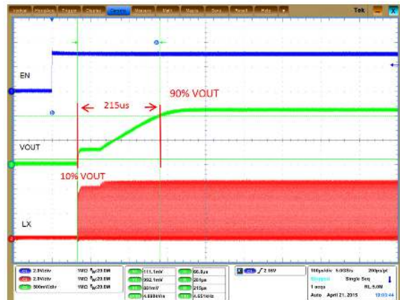
Figure 16. Soft-start Time for NCP6323D ( V_{IN} = 4.2\text{ V} , V_{OUT} = 1.1\text{ V} , I_{OUT} = 0\text{ A} , L = 1\ \mu\text{H} , C_{OUT} = 10\ \mu\text{F} )
