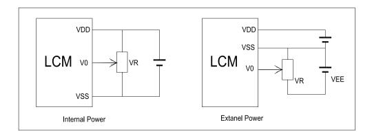
$V_{DD^{\sim}}V_0\text{: LCD Driving voltage}$
