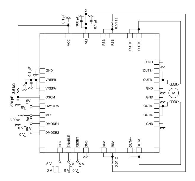
Note: I will recommend the addition of a capacitor if necessary. The GND wiring must become one point as much as possible-earth.
