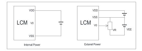
V<sub>DD~</sub>V<sub>0</sub>: LCD Driving voltage VR: 10k~20k
