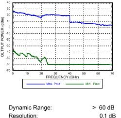
Power Accuracy:  $\pm 1 \text{ dB} > 500 \text{ MHz}$   $\pm 2 \text{ dB} \le 500 \text{ MHz}$   $\pm 2 \text{ dB} \le -20 \text{ dBm}$  (All Frequencies) RF OFF  $\le -90 \text{ dBm}$
