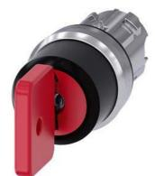
Key-operated switch O.M.R, 22 mm, round, metal, shiny, lock number 73037, red, with 2 keys, 3 switch positions I-O-II, latching, actuating angle 2x45°, 10:30h/12h/13:30h, Key removal I+O+II, with laser labeling, inscription or symbol Customer-specific selection with SIRIUS ACT configurator (CIN)
