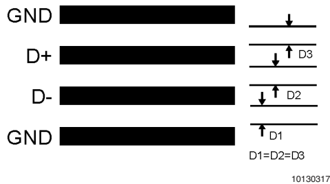
FIGURE 15. Ideal Diode Trace Layout
