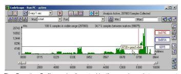
The Execution Profile graph allows to identify procedures that are executed frequently so that they can be optimized to gain system performance.
