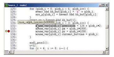
H/W breakpoints and S/W breakpoints (identified by red dots) may be used to stop execution in the critical code sections to allow detailed inspection of the embedded system.
