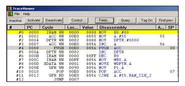
All **IRAM**, **XFR** and **XDATA** transactions in trace contain the **Value** read or written and the **address**. A separate columns for **Accumulator** (A) and **Stack Pointer** (SP) show the exact values as soon as they are changed.
