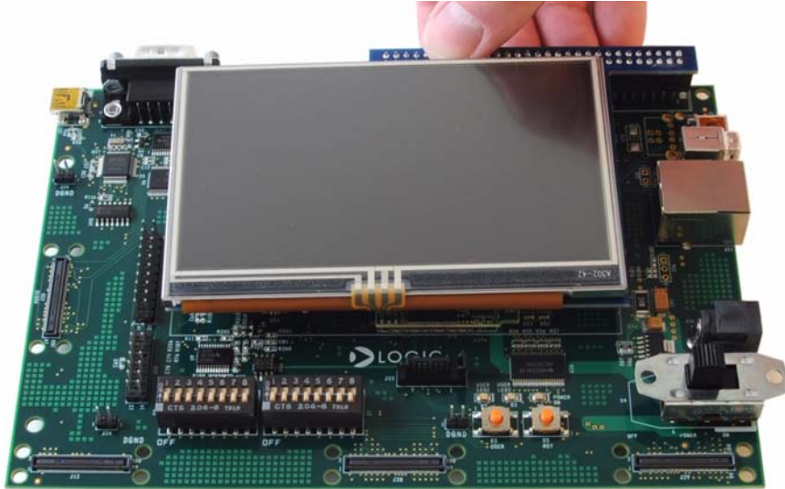
Figure 2.3 – Connect LCD to Baseboard
