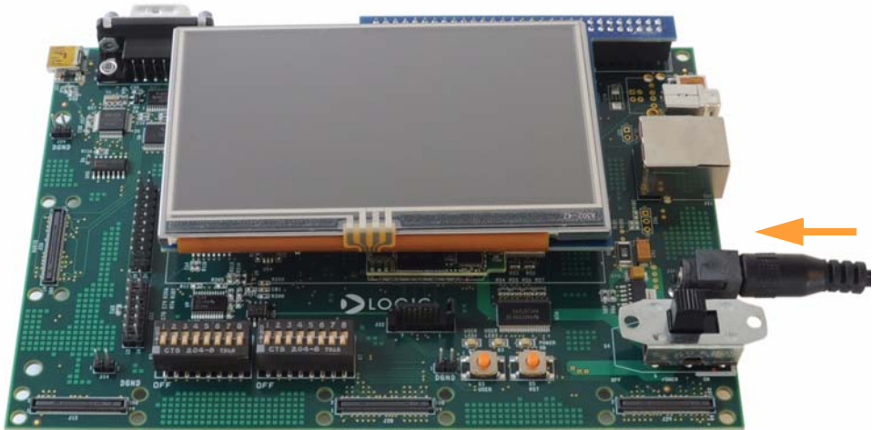
Figure 2.7 – Connect Power to the Baseboard
