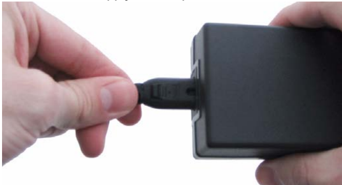
Figure 2.6 – Connect Power Supply and Adapter
