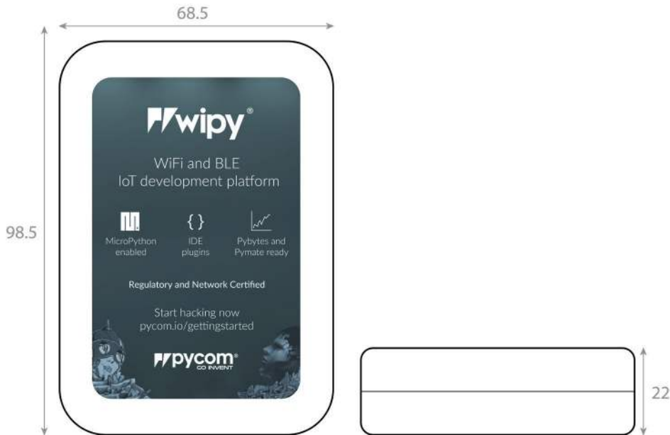
Figure 10 – Mechanical drawing of packaging – Units: mm
