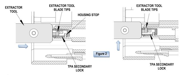
4. When the TPA is engaged, gently pull the extractor tool in the arrow direction shown, maintaining a constant pressure on the Extractor tool handle until the Secondary Locking Key (TPA) stops. When it stops the TPA is unlocked. Do not pull the TPA out of the connector. See Figures 3.
