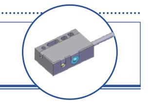
The OPB720 is a reflective switch designed to detect objects as far away as 24" (610 mm). Detectable object sizes can be as small as 0.08" (2mm) at a distance of 8" (20 mm). The OPB720 has a logical output that switches from a high level with no reflection target to a low level with a reflection target. With the addition of hysteresis, the OPB720 minimizes switching oscillations on the output. The open collector output transistor and power requirements is compatible with most PLC's
