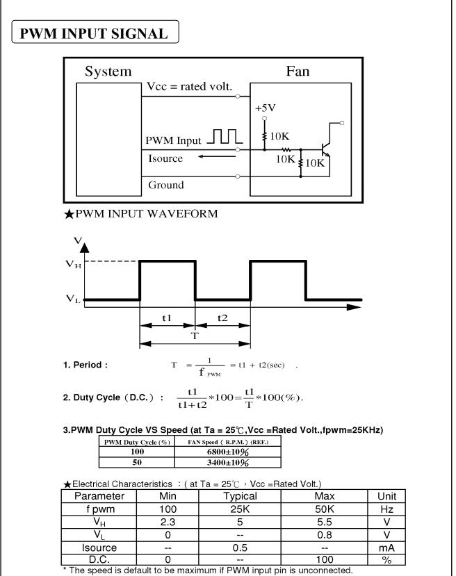
\* Min. start up duty cycle is 15%. Please don't apply 1 ~ 14% duty cycle to prevent unstable fan speed.
