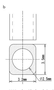
\* Nozzle with chamfering is recommended
