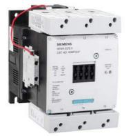
Vacuum NEMA contactor, Size 6, Three phase full voltage, Contactor amp rating 540A, 3 wire (NO aux included), 575-600V 50-60Hz/DC coil, Non-combination type, Enclosure NEMA type (open), No enclosure
