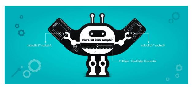
The **micro:bit Click adapter** comes comes equipped with two proprietary mikroBUS<sup>M</sup> sockets, allowing all the Click board<sup>M</sup> devices to be interfaced with the micro:bit with no efforts at all. It is enough to place the small standardized add-on board of your choice on the top of the mikroBUS<sup>M</sup> socket - and click it in. That is why this small add-on board is called Click board<sup>M</sup> - it just clicks!
